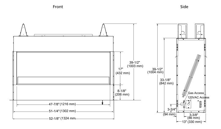
3" minimum under appliance. 6" minimum under appliance with optional drain pan (ODLANAIGST-48DP)
