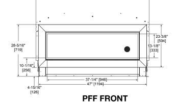
The PFF decorative front has an installed depth of 3/4" [19mm], measured from the front of the non-combustible finishing material to the front of the decorative front.
