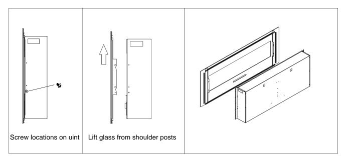
3. To replace the glass, lift onto the 4 shoulder posts. For a Wall Mount installation,replace the two or four screws to secure the glass. For Flush Mount installs it is not possible to replace the screws.
