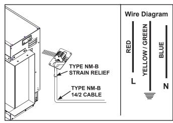
Figure 4.11 Wiring Diagram
