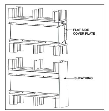
Figure 4.7 Flat Side Cover Plate
