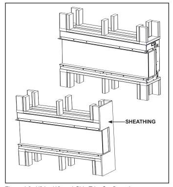
Figure 4.6 1/2 in. (13 mm) Side Trim Configuration
