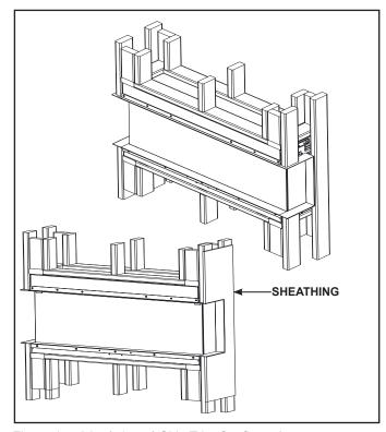
Figure 4.5 2 in. (51 mm) Side Trim Configuration
