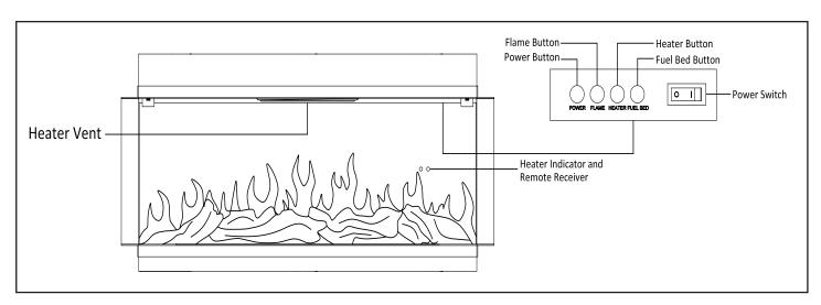
Figure 5.1 Manual Operating Switches and Indicator Lights
