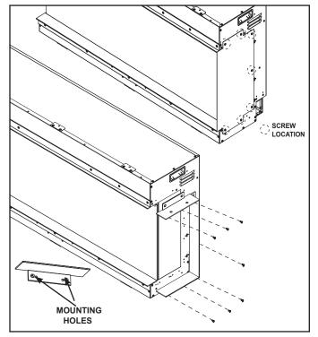
Figure 4.3 Plate Removal and Trim Install
