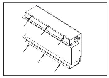
Figure 4.4 Mounting Brackets
