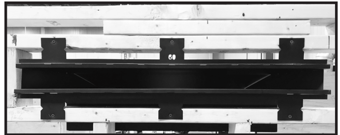
Figure 5.20 Plenum Secured in Place
