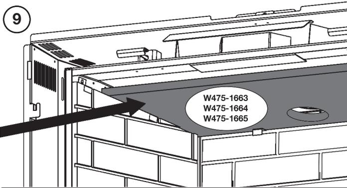
Install fibre baffle. It sits on top of the left and rear panels.
