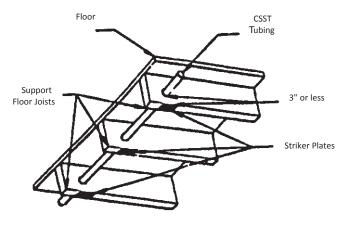
Figure 4-18 CSST Tubing Going Through Joists Within 3" of Potential Nailing Surface.
