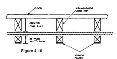
within a Wall Partition. Shielding Required at Support Area (studs) when
