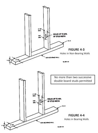
The size and depth of installation clearance holes or notches for routing the tubing through wall studs and joists shall comply with the requirements of the local building code.
