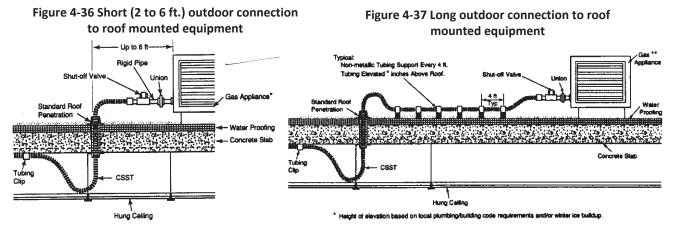
• Height of elevation based on local plumbing/building code requirements and/or winter ice buildup.
