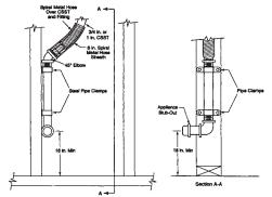
Figure 4-38 Appliance termination/stub-out
