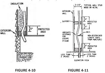
Long Unsupported Vertical Tubing Rugs (over 3 ft.) within a Hollow Interior Wall Partition. Shielding Required at Support Area When Points of penetration are Less than 2" From any Wall Surface.
