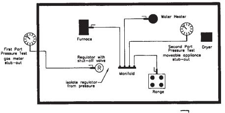
g) Most jurisdictions also require an additional pressure or leakage test performed after the construction is completed and finished interior walls are in place. The leakage test procedure is generally performed by the gas utility at the time of setting their meter. This test is performed to assure no damage was done to the tubing during the closing-in construction process, and is typically required before gas service is initiated.
