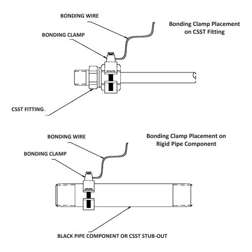
Depending upon conditions specific to the location of the structure in which the flexible gas piping system is being installed, including but not limited to whether the area is prone to lightning activity, the owner of the structure should consider whether a lightning protection system is necessary or appropriate. Lightning protections are beyond the scope of this guide, see NFPA 780, the Standard for the Installation of Lightning Protection Systems, and other standards.
