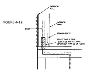
Where Finished Exterior Wall Does Not Permit Installation of Striker Plate, Protective Sleeve is Required.
