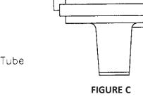
The regulator may be mounted horizontally, with a vent tube installed in the venting port. The end of the tube must be facing downward, and should be designed to prevent water and foreign material from causing a blockage.
