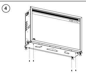
Mount the appliance onto the supporting plate. Use the 4 screws and screw holes from Step 3.
