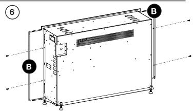
Install the left panel and right using the screws removed in Step 5.
