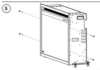
Remove the 2 screws on both the left and right side of the appliance. Set the screws aside.
