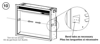
After completing the trim installation, we recommend having two people carefully lift the appliance into the finished framing. We recommend securing the appliance to the frame, using the bend tabs available on the appliance (see above). Continue the rest of the appliance installation (from step 6 of page 12 of appliance installation and operation manual).
