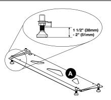
Pre-install 4 levelling feet and nuts into the support plate. Measure the levelling feet based on the height of the enclosure in your woodbox. Typically, the levelling feet are secured 1 1/2" (38mm) to 2" (51mm) from the appliance.
