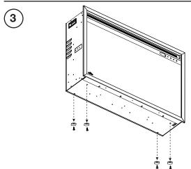
Remove the 4 screws with the rubber pads from the unit chassis. Set the 4 screws aside.
