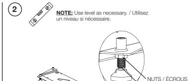
Level the support plate by adjusting the 4 levelling feet on the supporting plate. Afterwards, tighten the 4 nuts.
