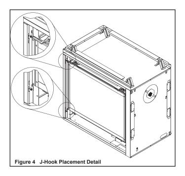
Install Decorative fronts on each side of appliance per instructions included with decorative fronts. Pull gently on both decorative fronts and end panel to ensure that J-Hooks are seated properly and securely on shoulder bolts. See Figure 5 and Figure 6.
