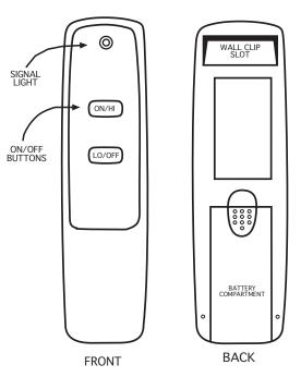
This remote control SYSTEM offers the user a battery-operated remote control to power a DC servo motor such as those used with gas valves used in some decorative gas logs, gas fireplaces and other gas heating appliances.
