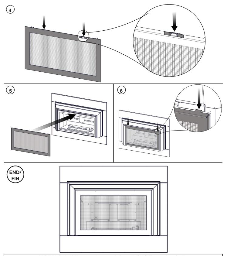
**NOTE:** Cleaning the safety screen may be necessary due to excessive lint / dust from carpeting, pets, etc. Simply vacuum using the brush attachment.
