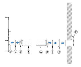
For a better seal, you may also use aluminum tape. Wrap the tape around the joint between the flexible pipe and the air inlets. Carefully push the insulation and plastic cover back over the pipe. Fix the plastic in place using aluminum tape.
