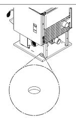
When installed in a mobile home, the stove must be anchored to the floor with two screws. Use the two anchoring holes located on each side of the pedestal, as shown on the right figure.
