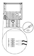
Open the thermostat and connect the wires as per the manufacturer's instructions.
