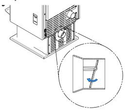
Test the door seal by closing and latching the door on a strip of paper. Test all around the door. The paper should not slip out easily. If it does, see the maintenance section in the operation manual.
