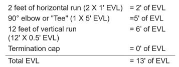
Since the total EVL is less than 15 feet, the recommended exhaust venting diameter is 3".
