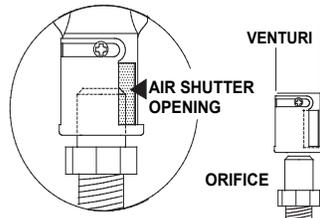
Closing the air shutter will cause a more yellow flame, but can lead to carboning. Opening the air shutter will cause a more blue flame, but can cause flame lifting from the burner ports. The flame may not appear yellow immediately; allow 15 to 30 minutes for the final flame colour to be established.
