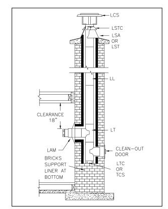
Fig. 7 – Existing masonry relining installation
