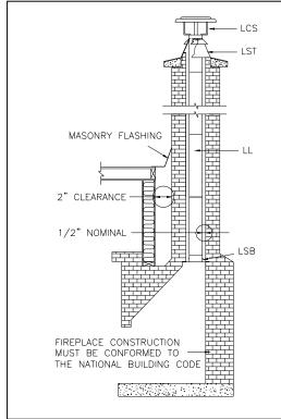
Fig. 8 – Lining system for new fireplace installation
