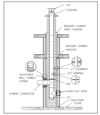
Fig. 4 – New masonry liner installation for interior chimney
