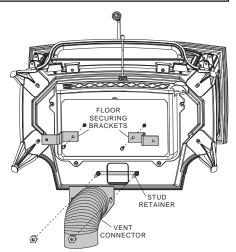
Secure the vent connector in place using the 2 nuts supplied.
