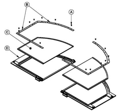
It might be necessary to replace the glass gasket from time to time. The gasket is flat, adhesive-backed, woven fibreglass. Remove the glass retaining screws (A) and the 4 metal frames (B) that hold the glass (C) to the door frame (D). Lift out the glass (C) and pull off the old gasket. Do the same for the other door. This is a good time to clean the glass thoroughly.
